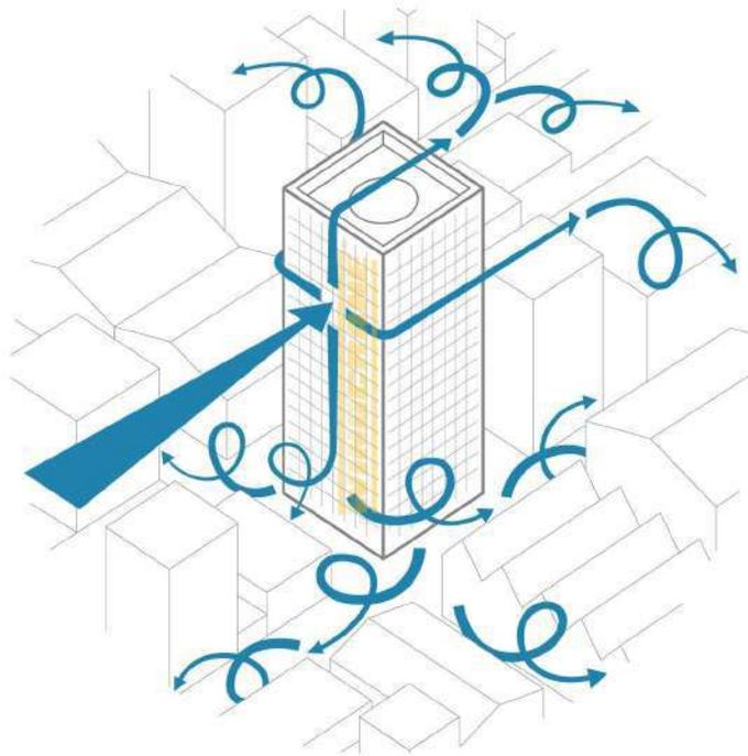
*Figure 7: The Effect of Wind Flow On a Building Located in A City (Source: WindCrane)*
