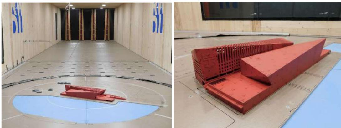
*Figure 14: Model of the Royal Caribbean Cruise Terminal in the Boundary Layer Wind Tunnel (Source: RWDI Consulting Engineers)*
